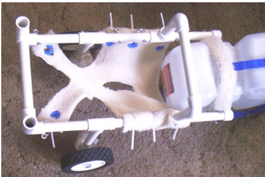
**Sling.** This material must be sturdy, non-stretching, and non-raveling, yet comfortable on one side against the dog's delicate belly skin and groin areas. I found
