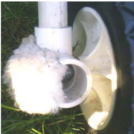
**Attaching harness to frame.** Build the rest of the frame first so you can adjust the harness attachment point. Drill a hole for each eyebolt right behind the cap end of the PVC (remember, at an angle so they don't rub against dog's side) then screw in and attach the nut. Sew any sturdy nylon strap material onto the harness and a hook with sturdy thread, dental floss is excellent. Pieces cut from a nylon puppy or cat collar would work well for the strap.
